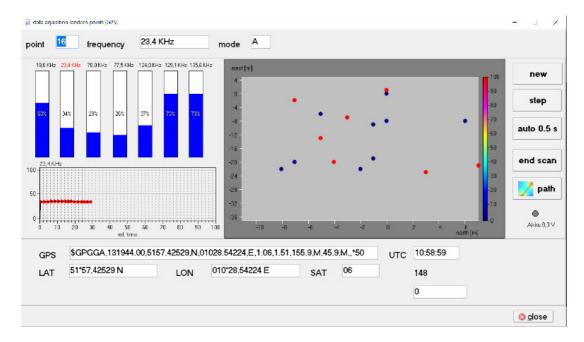
The corresponding coordinates are provided by the integrated GPS receiver. Manual triggering at the individual measuring points or measurements in a selectable time grid are available.
