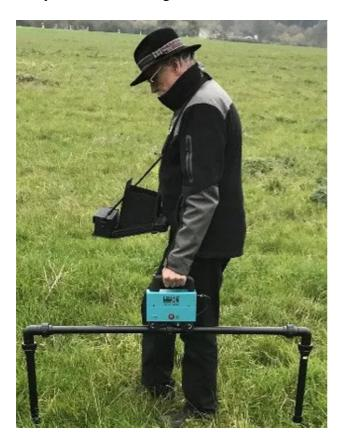
The previous time-consuming measurement in a fixed measurement grid has been extended by a GPS-supported, random measurement method.
