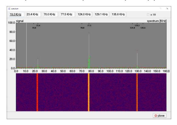
Depending on the reception situation, existing long-wave transmitters or the frequencies of the user's own generator can be selected.
