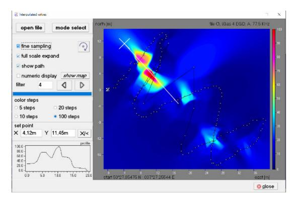
Different filters can be selected and a synthetic profile (white line) can be determined. For easier orientation, the direction and distance to points of particular interest can be determined.
