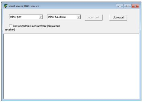
After starting the program the COM port and the baud rate must be selected in two combo boxes. Afterwards the button [open port] is released. A click on [open port] opens the connection. Central element is a field with 26 elements for float numbers (corresponding to A ... Z), in which transmitted values (parameters) are stored.
